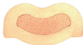
B Crimp on Flexible Copper Cable
