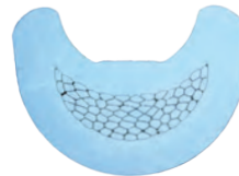
Deep Indent on Aluminum Cable for Aerospace Industry
