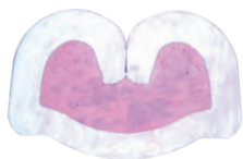
Open Barrel Connection Crimp
